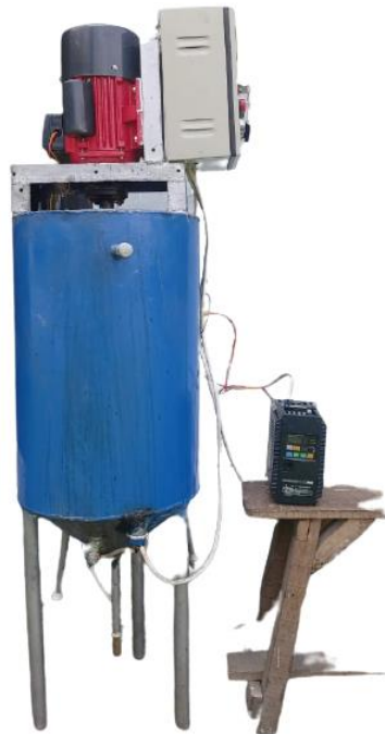
Gambar 1. Continuous Settling Tank
